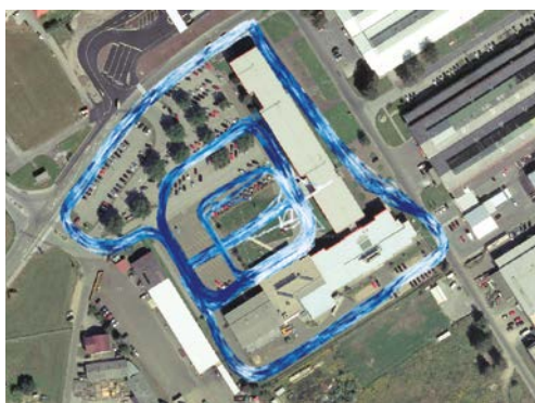
Figure: Differences in asphalt quality at the JOANNEUM Technical College Campus in Kapfenberg (dark blue = poor)
